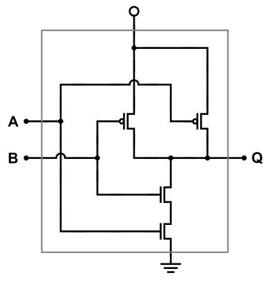
We can replace the circuit within the box with the following NAND symbol. Note that there are 5 connections (just like in the box above):
